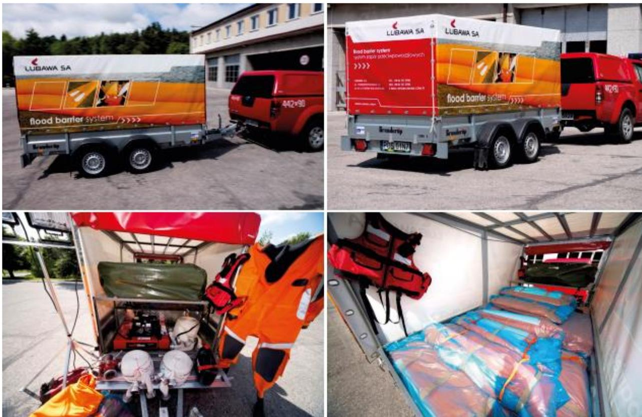
Trailer for flood rescue is intended to carry out flood action with the equipment contained in it: flood barriers filled with water FB3L, manufactured by LUBAWA S.A. On the trailer there are all the tools and equipment necessary to position barriers in different area and weather conditions. A trailer can be ordered in several versions – in different capacities and sizes, to meet the customer's needs, as well as to the vehicle, by which is to be transported.
