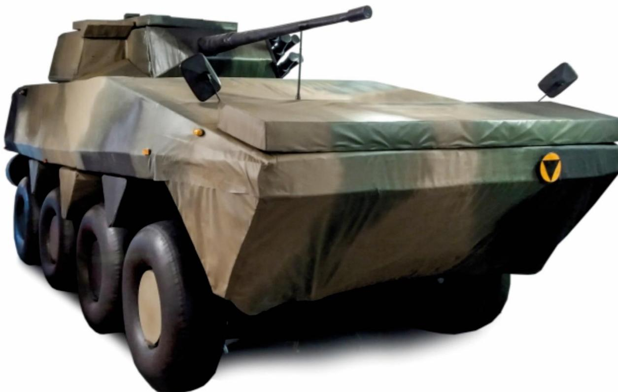
Decoys are designed to mislead an observer from actual targets and to misrepresent the actual number information of deployed forces. Decoys also serve targets for training operation and live fire exercises. The product presented shows the technological and construction possibilities available.
