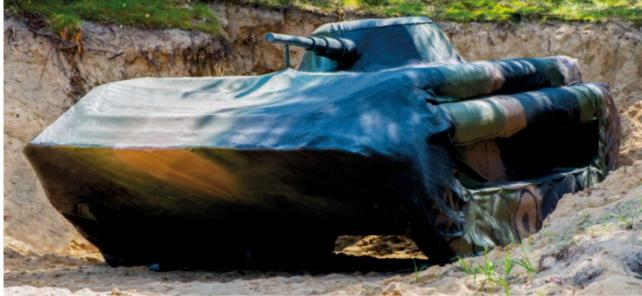
The inflatable mockup is designed to simulate individual objects or groups of equipment in mixed (mockups and real equipment) or simulated (only mockups) conditions. Inflatable mockups simulate the presence of the equipment in a wide spectrum of electromagnetic radiation used in the reconnaissance, i.e. in the visible, thermal and radiolocation range.
