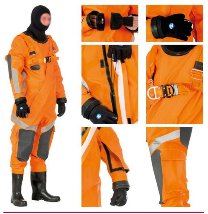
Suit for water-work is made of polyester fabric coupled with polyester knit, with water-proof zipper, neck seal, hood and permanently fixed rubber boots. It protects the whole body against getting wet.
