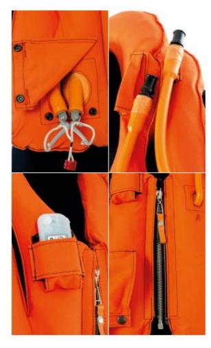
Pneumatic lifejacket with automatic filling system deploying when immersed in water to a depth of 10 cm. Another advantage is the possibility of inflation by mouth. Temperature range -30°C +50°C. Vest is able to maintain user on surface of water by min. 6 hours.
