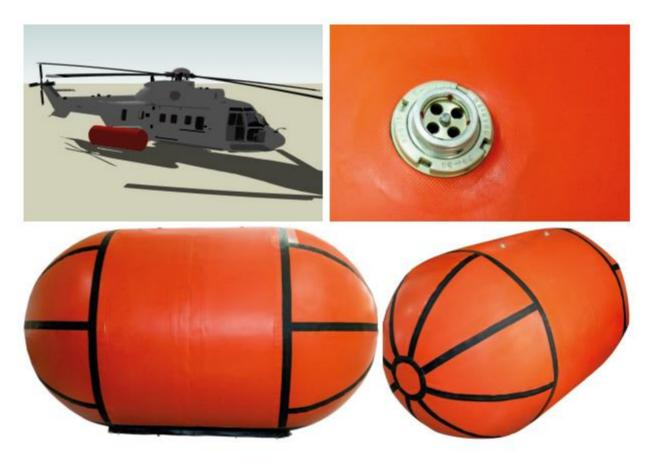
Pneumatic floats are made of rubberized fabrics which are fixed to the helicopter's body; their function is to quickly open from the cover and, after quick filling, to keep the helicopter on water surface, enabling the crew and the passengers to get to life rafts after ditching.
