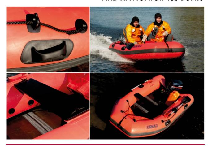
The stern of the Orka and Orka 2 pneumatic boats is equipped with a permanently glued wooden transom for mounting an outboard, electric or internal combustion engine with a short engine leg. The boat has four independent air chambers that guarantee its completely safe operation. The Orka and Orka 2 boats can be equipped with a fully-folded wooden floor or with an Airmata-type pneumatic floor and a pneumatic keel that profiles the bottom and guarantees full comfort.
