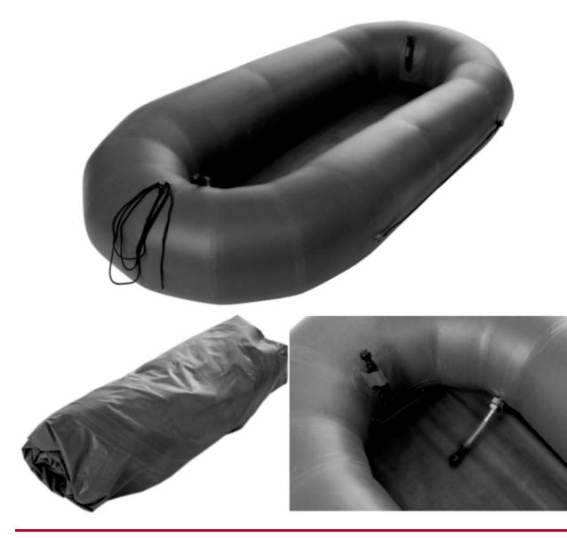
A pneumatic inner tube of the boat has a 4-compartment design. It features inlet- outlet for tubing for filling the compartments with air, and flow tubes for distributing the air between the compartments. Clamps are attached to flow tubes to close the air flow between the compartments. The basic (abridged) version of the instructions for use is placed on the dinghy's inner side of the bottom. The bottom is permanently fixed to a pneumatic inner tube.
