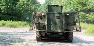
The system is exceptionally lightweight – the net and profiles alone weight only 4.75 kg/m2. The weight of the entire panel depends on the shape and size of the frame. The product is subject to the EPO / PCT patent procedure, patent application ID EP19461550A.
