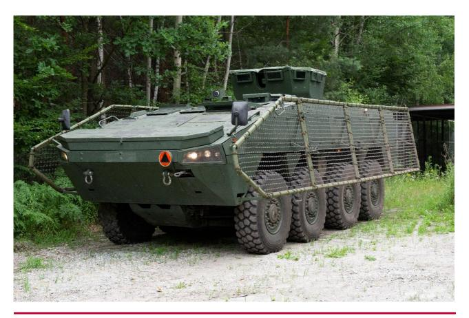
The lightweight RPG net screen is designed to protect vehicles and other military objects against impacts from PG 7W and PG 7WM type High Explosive Anti-Tank (HEAT) grenades. The system is composed of individual net modules tailored to the size and dimensions of the object to be protected.
