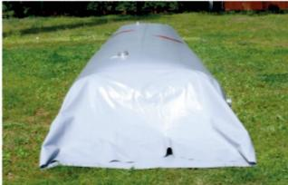
Water filled high-water flood barrier are an alternative to flood barriers built with sandbags. The flood barriers form a closed water basin. They are made of a 3-layer, PVC-coated watertight fabric. This makes them particularly resistant to long-term effects of water, air and UV radiation. The materials used make the flood barrier reusable. The flood barrier is used to build or heightenflood banks.
