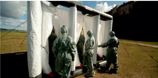
The inflatable PVC cabin is designed for cleaning, disinfecting and decontaminating protective clothing contaminated with chemical substances. Three decontamination lines (cabins) allow for very quick operation – up to 3 persons can be decontaminated at the same time.
