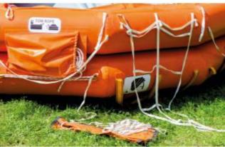
High seas airborne inflatable raft is designed for rescue operations in life-threatening situations at open sea. The raft is made of rubberized textile with good resistance to ageing, high resilience to wear and rupture, resistance to low and high temperatures, UV radiation, marine weather conditions.
